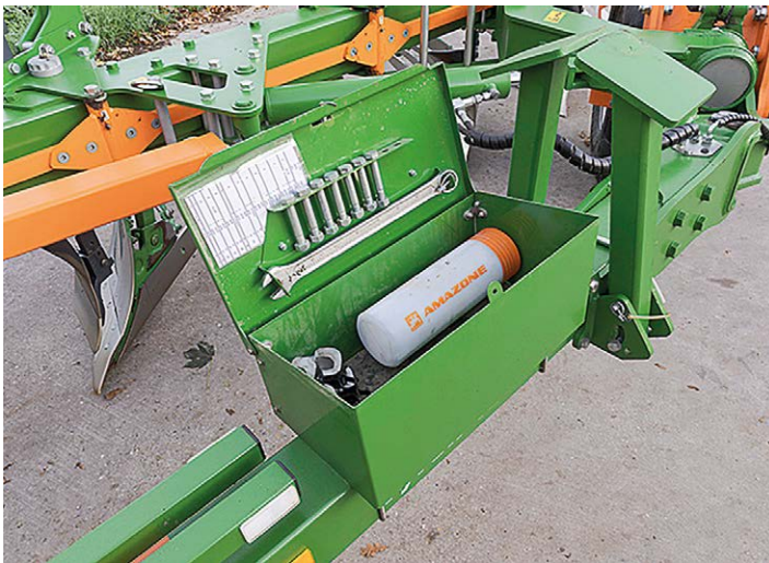
The sturdy box stores tools and other essentials (left). A 24/30 spanner is supplied with the machine. Not all of the grease nipples are easy to reach.
