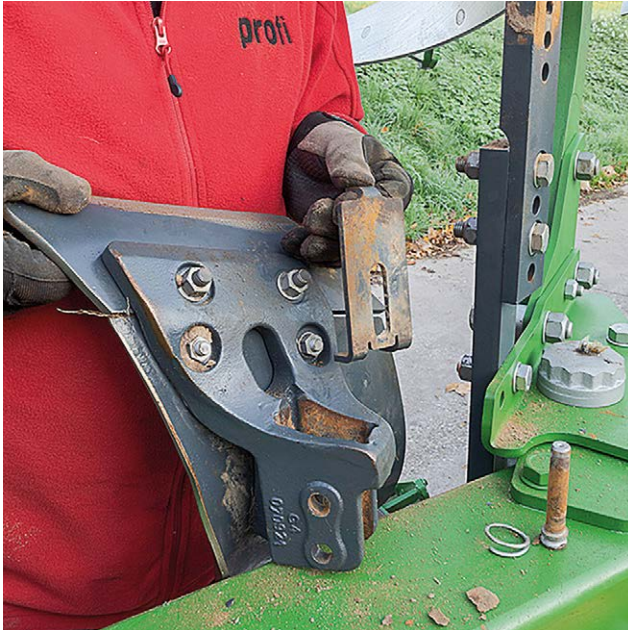
The depth and skimmer over/underlap can be adjusted by repositioning the plate (left). The disc in its far forward position didn't block once.
