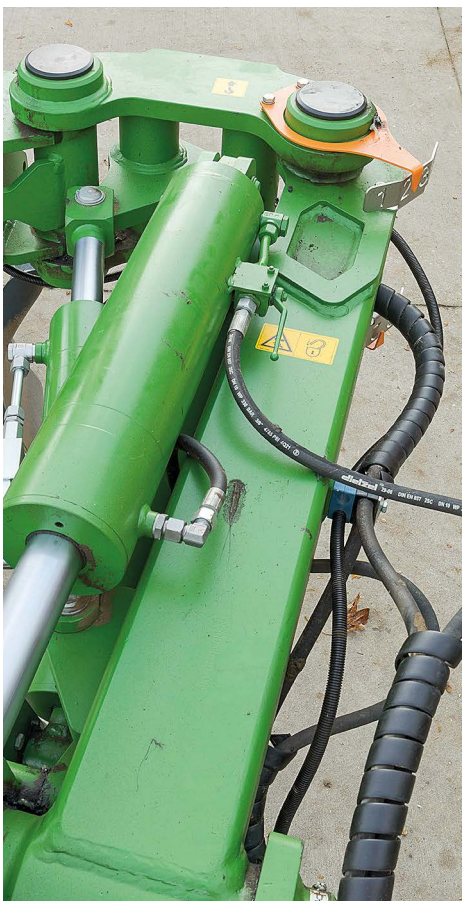
Three settings are changed hydraulically on the Tyrok 400V: front furrow width (left), depth (upper right) and working width (lower right). Operators have little cause for complaint on the setting options.
